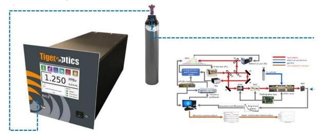
SUN validates and performs an inter-comparison of the CC-FS-CRDS spectrometer using a reference humidity generator. SUN, with the support of INRIM, assesses the performance, potential effects of gas matrices on the measurements, and measurement uncertainties of the CC-FS-CRDS spectrometer in the amount fraction range between 5 parts in  $10^6$  (5 ppm) and 5 parts in  $10^9$  (5 ppb) with relative standard uncertainties between 3% and 8%, from the upper to the lower range, respectively.
