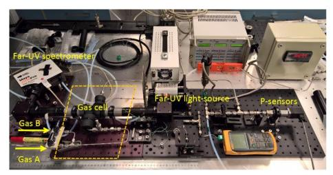
DTU is developing a compact and transportable far-UV system for trace water vapor measurements in Ar,  $N_2$ , and  $H_2$ , ranging from 5 ppm to 5 ppb, with a standard relative uncertainty between 3% and 8%, and an operating pressure of up to 1 MPa.
