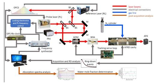
SUN is developing a compact NIR CC-FS-CRDS spectrometer to enhance sensitivity, thereby reducing the limit of detection. This spectrometer is referenced to an optical frequency comb for traceable measurements of water vapor in  $H_2$  and  $N_2$ , ranging from 5 ppm down to 50 ppb, with a standard relative uncertainty between 3% and 8% and an operational pressure as low as 10 kPa.
