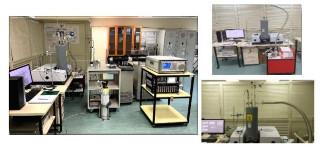
TUBITAK is improving the existing FTIR-based trace water measurements in N2 and Ar from 5 ppm to 50 ppb with a standard relative uncertainty between 3% and 8% and an operating pressure of up to 1 MPa. The existing high-resolution FTIR system is being upgraded with a new pump system and a new multi-pass gas cell to enable water vapor measurements down to 50 ppb and operating pressure in the cell of up to 1 MPa.
