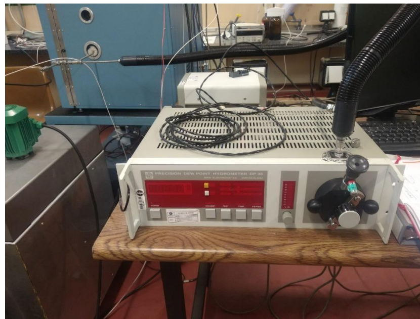
Dew point hygrometer, MBW, DP 30 model
