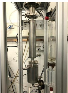
VTT Permeation system based on a passivated magnetic suspension balance
